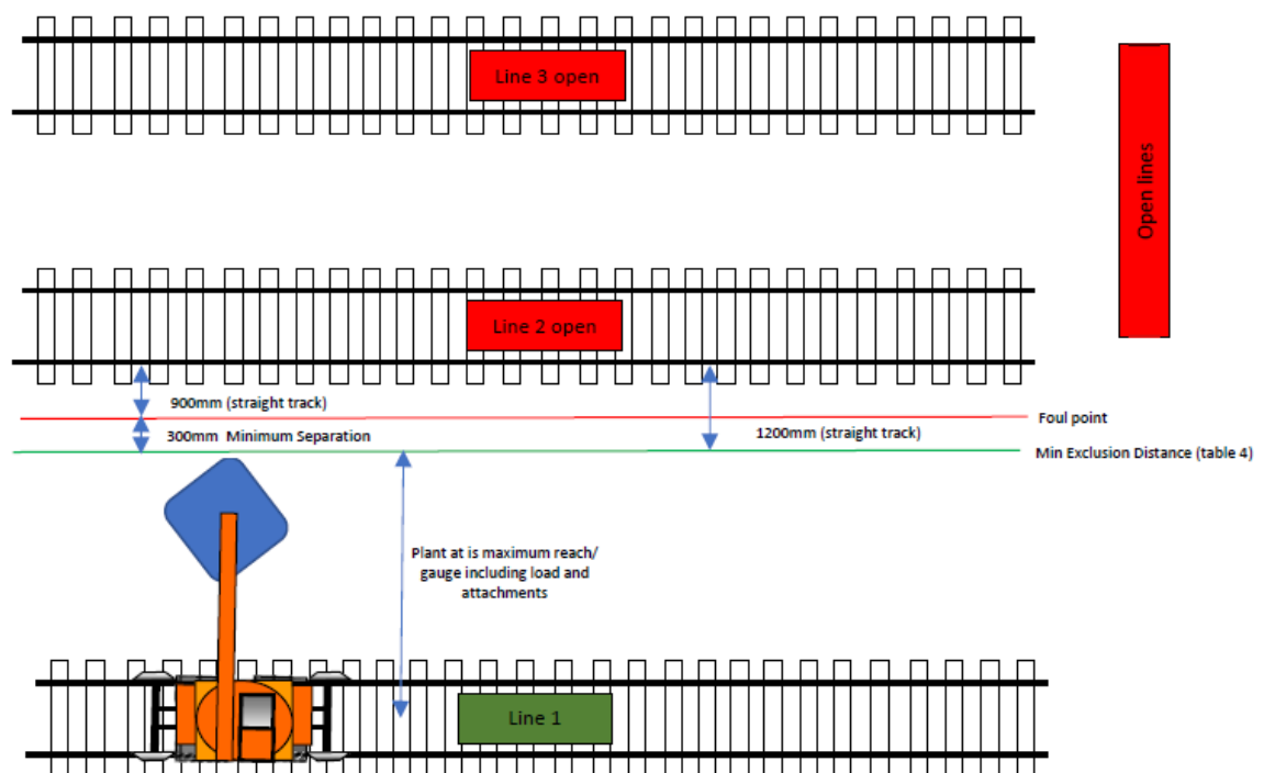
Figure 1a Diagrammatic view of plant working that cannot foul (rail)
